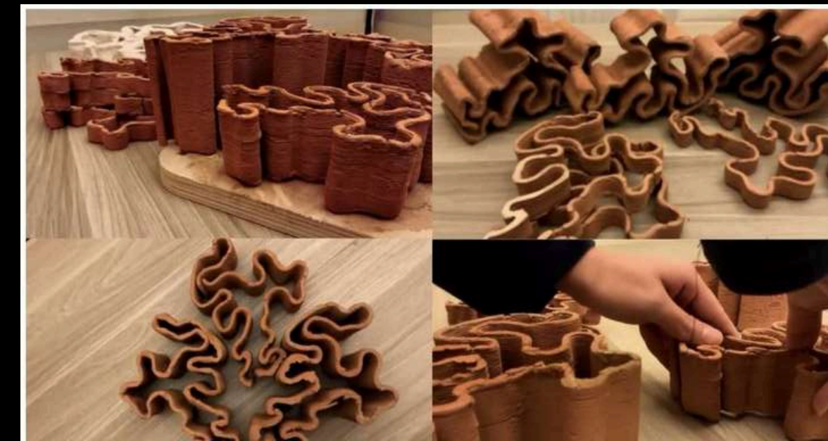
Fired terracotta — post-kiln 1000–1200°C, ready for testing
