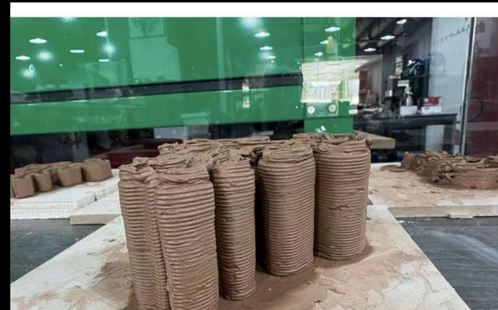
Clay colour shifts as moisture evaporates during drying
