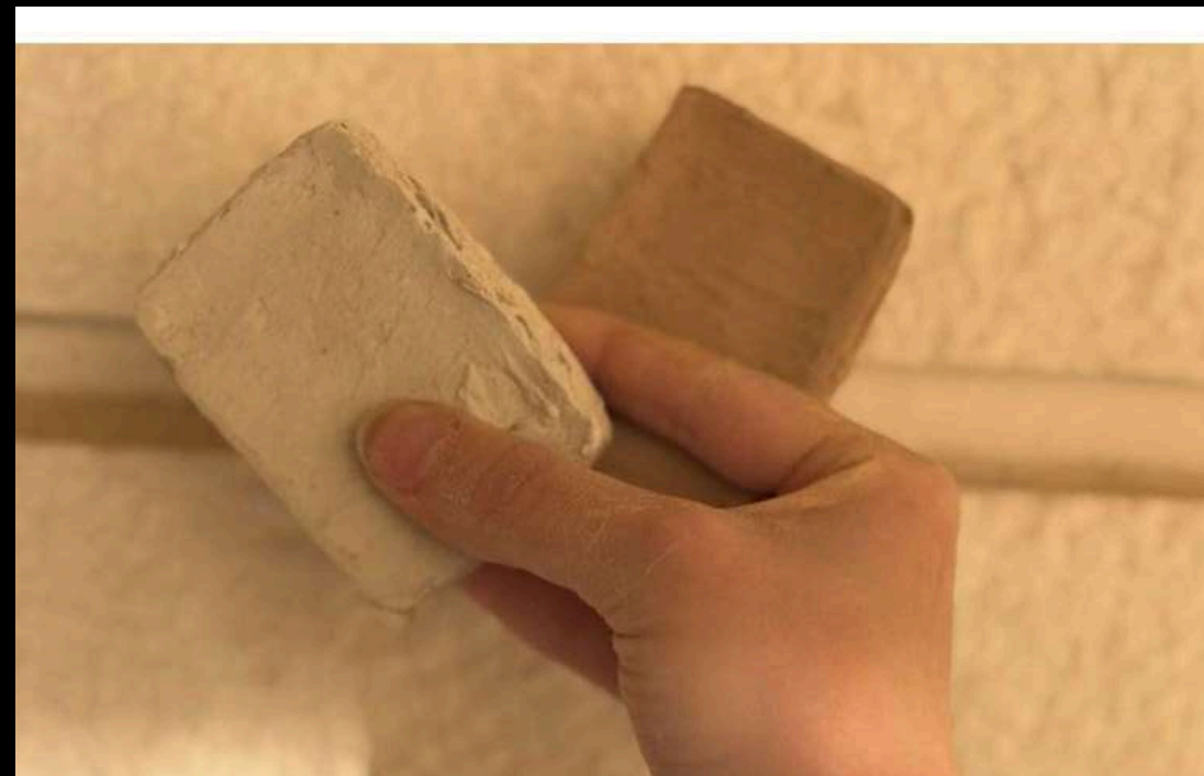
Local Jordanian clays — Dhana (left) and Irbid (right), tested for printability
